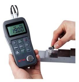
modes: Single point mode and Scan mode; Coupling status indicator showing the coupling status; Auto sleep and auto power off function to conserve battery life.
